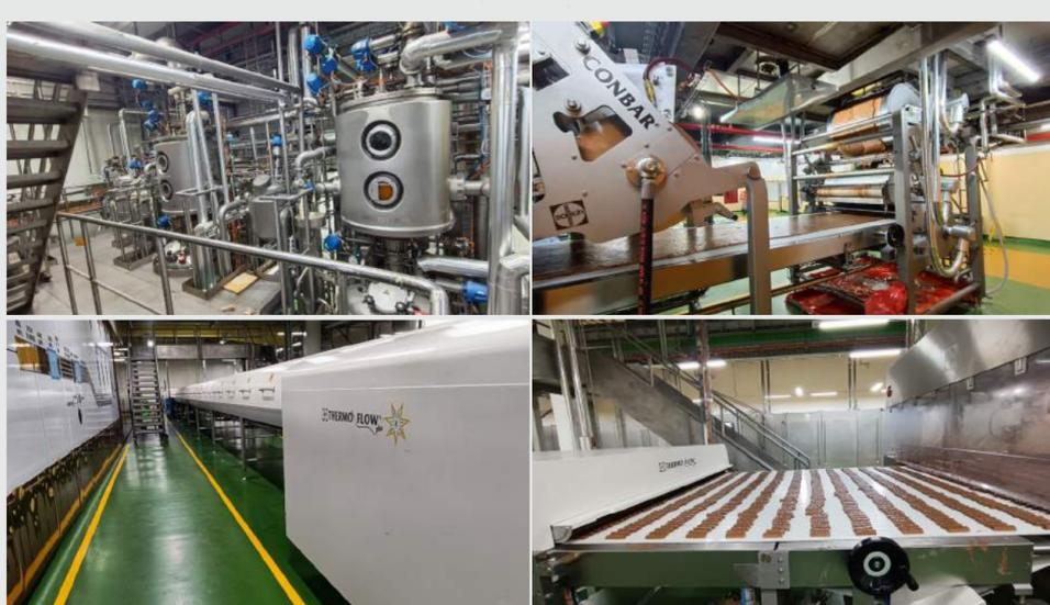
Shaping/Forming of the bar is done using the **Sollich Conbar®**, a line which is also suitable for forming other products made from fatty masses, soft boiled sugar masses, aerated fatty and sugar masses, and a wide variety of mixtures containing nuts, fruit, and cereals.
