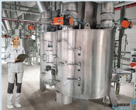
The solution: **The amixon® HM 2000 twin-shaft mixer**
