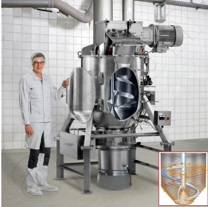
finished mixture flows from the mixer through the mixer outlet bin directly into the packaging machine. Cleaning work is greatly reduced because this mixer empties residue-free.
